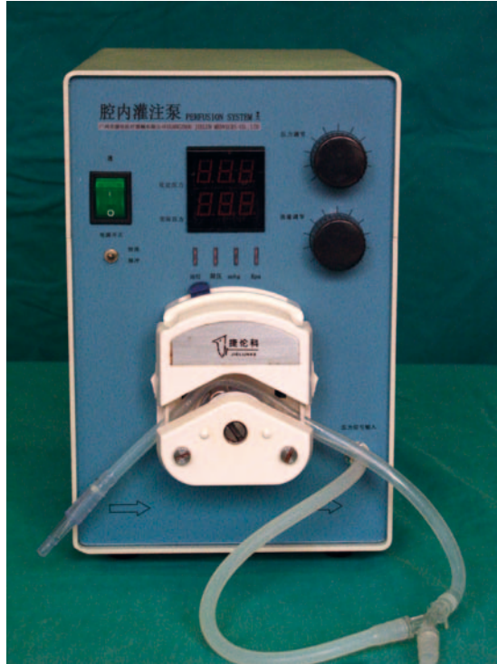
Figure 2 Specially-designed pump for mini-PCNL China.
