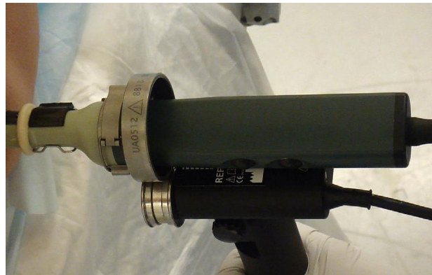
FIGURE 2.I-11 Transrectal Probe Attached to a Magnetic Rotation Holder During Data Acquisition
